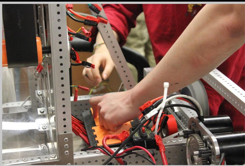
**Electronics, batteries, and wires are installed and tested by students and then the controls team programs the robot with java, as well as testing and refining visual controls.**
