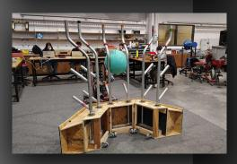
In order to test and practice driving the robot, the team has recently been working on making a completed version of the field element called the Reef. This week, new welded metal reef segments were made by Mike, our mentor from Frontline Bioenergy, which made the reef a lot more reliable and game accurate.
